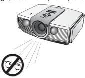
Do not operate the projector lamp beyond the rated lamp life. Excessive operation of lamps beyond the rated life could cause a lamp to break on rare occasions.
